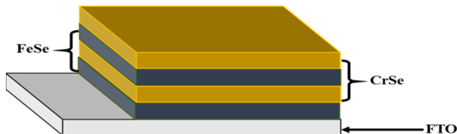
Figure 2. Diagrammatical representation of FeSe/CrSe superlattice formed by electrodeposition.
