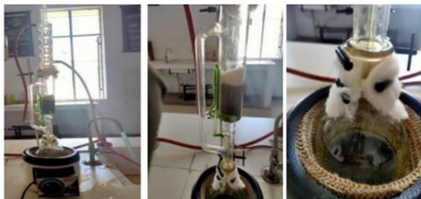
Figure 3. Soxhlet Assembly showing extraction process.
