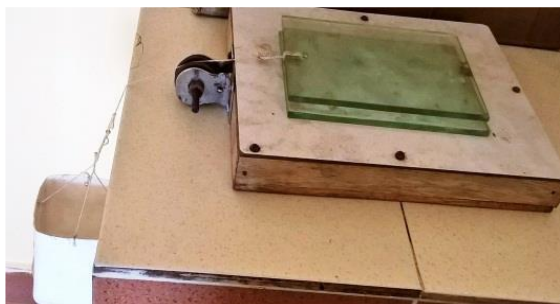
Figure 1. Shear stress apparatus for determination of mucoadhesivity of isolated biopolymer
